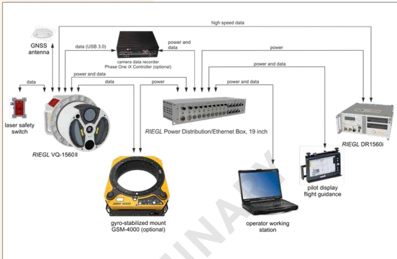
A minimum number of system components and external cabling is required for an easy and quick installation in aircrafts.
